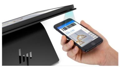
Camera based barcode scanner\* is behind the top corner of the display \*Appropriate software drivers required
